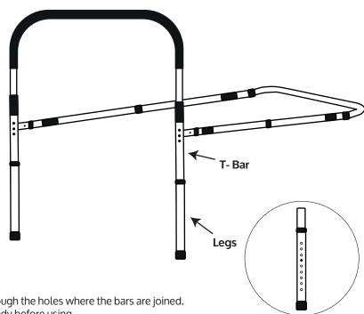
Before use, check that all push-pin buttons fully protrude through the holes where the bars are joined. Ensure both legs touch the floor and that the hand grip is steady before using.
