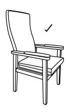
Lay the wood frame on its side so you can access the screw holes. Align the back with the wood frame and use the screws provided to attach the back to securely to the wood frame (make sure to use the M6 x 40mm screws on the back of the chair and the M6 x 30mm screws on the front of the chair). Put the chair upright and place the seat cushion on the chair and enjoy your Vitra Fireside Chair.
