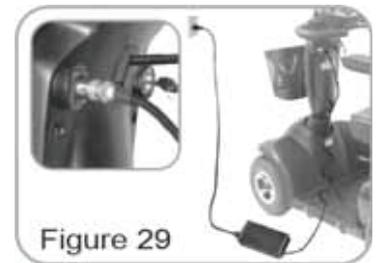
1. Insert battery charger cord into the charger connector on the charger output. Refer to above figure for correct position
